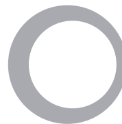
Cross section of a cold drawn tube with variations in wall thickness
