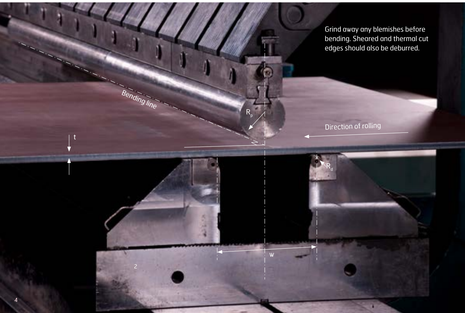
FIGURE 1 Bending transverse to the direction of rolling.
