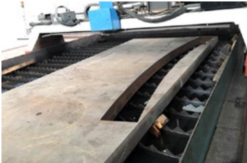
Fig 1. Oxycutting of Toolox® piece
