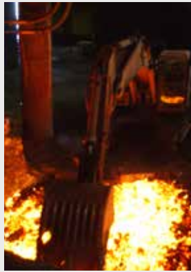
Buckets made in Toolox® 44 can take both wear and heat when handling red hot slag without losing its properties.
